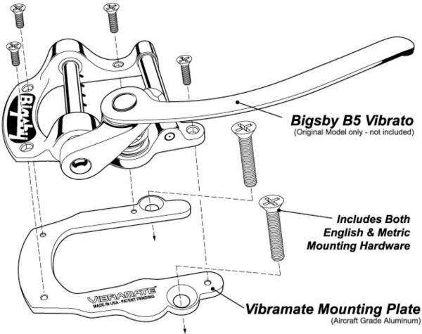
The Vibramate V5 Model Quick Mount Kit is designed for a Bigsby B5 Original Vibrato and will fit most traditional style guitars that have a tune-a-matic style bridge and a stop-tailpiece. The kit installs in minutes with the included hardware and eliminates the need for drilling permanent holes in your instrument. Be sure to follow the mounting instructions to prevent damage to your instrument. The Vibramate Quick Mount Kit includes both English and Metric threaded hardware.
